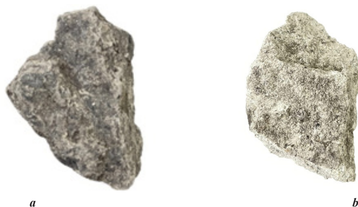
Fig. 2. Overburden rocks of the Ekibastuz coal basin: a - mudstones; b - siltstones
